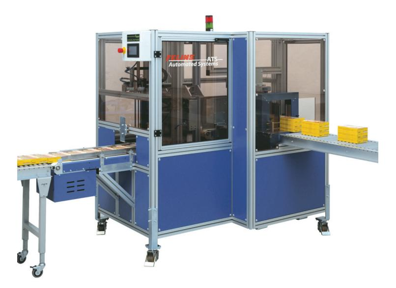
The US-2000 Stacking, Collating and Banding systems will accumulate from a single stream infeed. Stack counts are selected by the system operator. Orientations of 2 x 3, 3 x 3, 1 x 6 are common. The band eliminates the need for inner cartons. Product specials and multi-packs are processed at packaging line speed while minimizing labor requirements. Printed banding material can be used for product identification and multi-pack coding.
